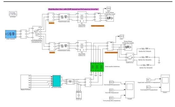
Figure 5. Distribution line model with DVR based on Embedded Z source inverter
