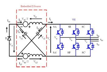
Figure 2. Embedded impedance (Z) source inverter
