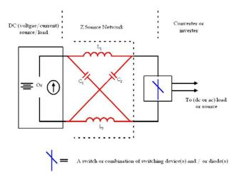
Figure 1. Impedance (Z) source inverter
